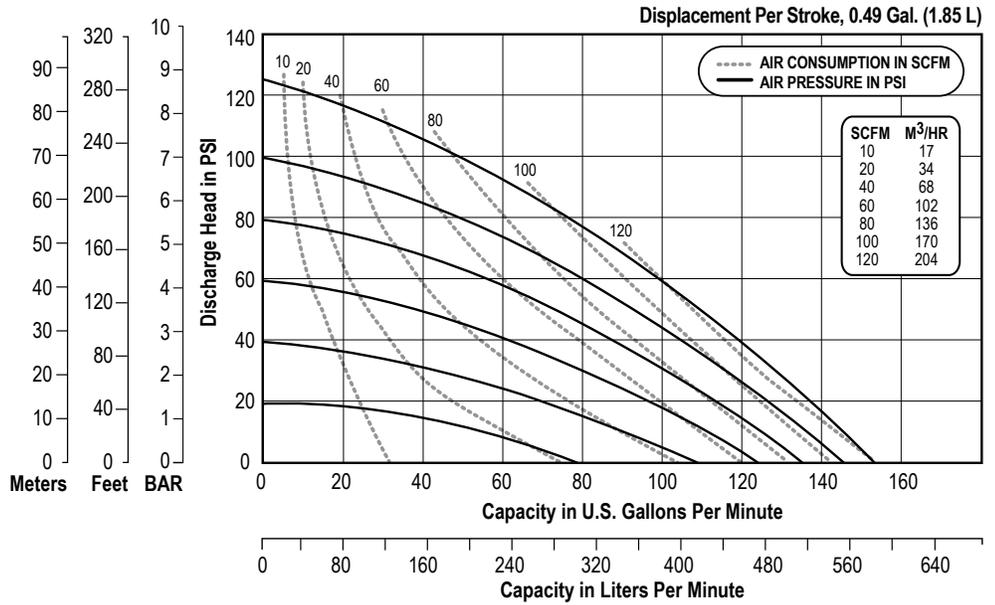
NOTE: Performance based on the following: elastomeric fitted pump, flooded suction, water at ambient conditions. The use of other materials and varying hydraulic conditions may result in deviations in excess of 5%.
