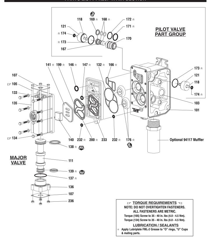
A replacement Major Valve Service Assembly is available separately, which includes the following: 637374 for models PD20P-X: 105 (4), 107 (2), 111, 132, 135, 136, 137, 138, 139, 140, 141, 146, 147, 166, 176 (2), 199, 200, 232 (2), 233 and 236 (4). 637374-1 for models PE20P-X: 76, 105 (4), 107 (2), 111, 132, 135, 136, 137, 138, 139, 140, 141, 146, 147, 166, 176 (2), 199, 200, 232 (2), 233 and 236 (4).
